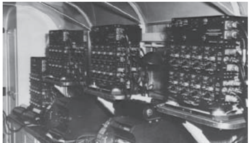
Amplifiers and recording oscillographs in bridge trailer.
