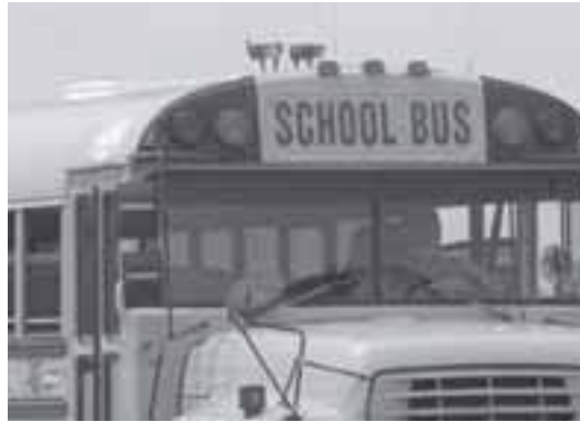
Antennas mounted on top of ISD school buses function as part of radio communication and AVL.
