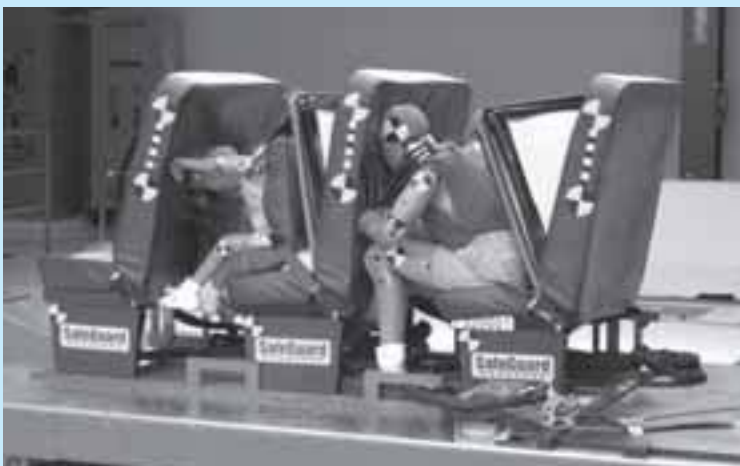
Sled test of "seat within a seat" design (SafeGuard's SmartFrame) gauges effectiveness of lap-shoulder restraint for buckled students, as well as extent of maintaining protection for unbuckled students.
