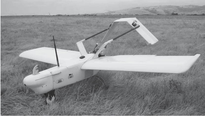
Mini-UAV bat or drone ready for take-off. Launching can be by hand or by lightweight bungee-powered catapult.
