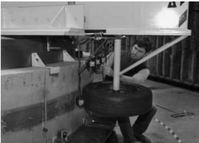
Purdue apparatus can test a range of tires and pavements, isolating the causes of highway noise.
