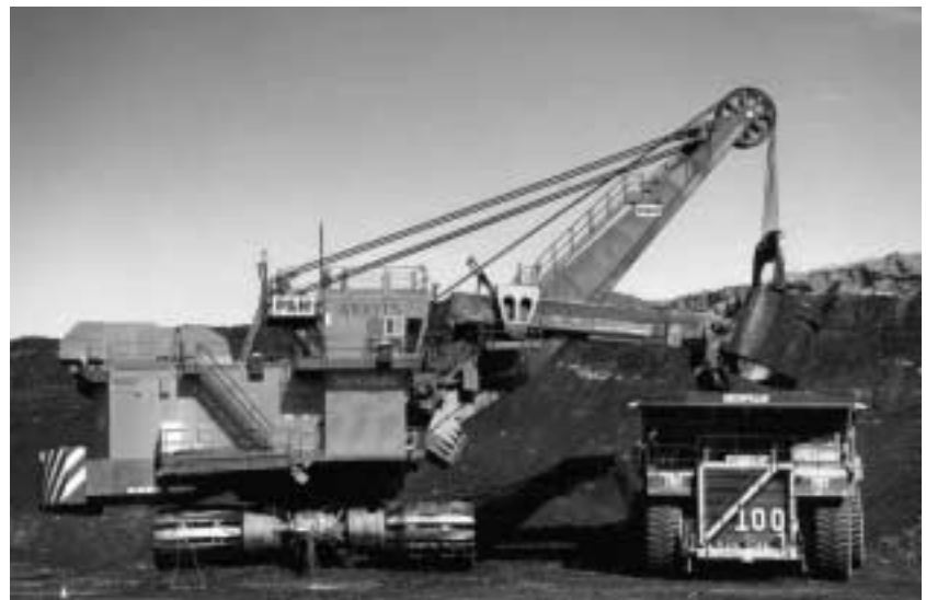
Electric cable shovel loads Canadian oil sands into hauling truck.
