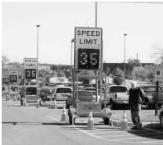
Maryland State Highway Administration demonstrates variable speed limit system to be deployed in summer 2003.
