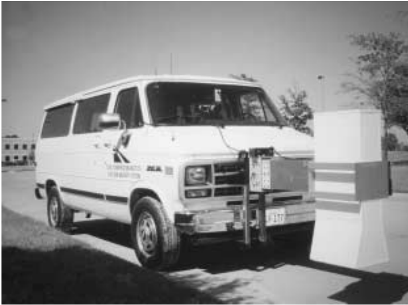
Texas DOT is preparing to train personnel from other state agencies in the use of ground-penetrating radar units, with help from Texas Transportation Institute.
