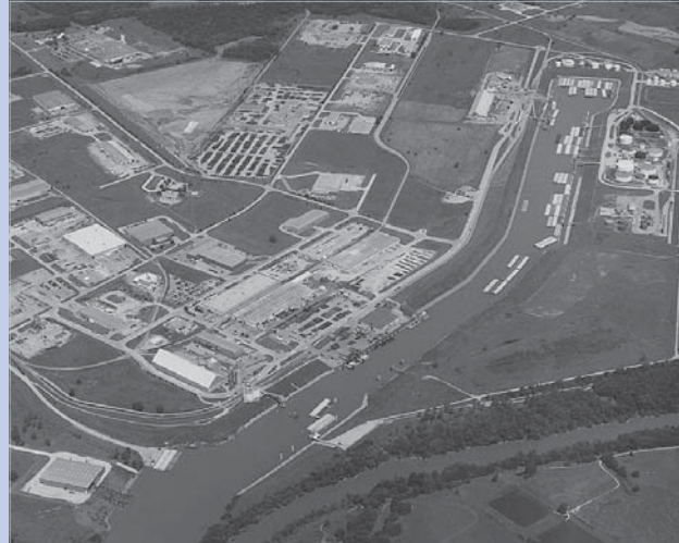
Aerial view of Tulsa Port of Catoosa, an excavated "slack water port" with no inlet, filled with backwash from Verdigris River at lower right. After joining the Verdigris, vessels from port travel 50 miles to connect with Arkansas River.
