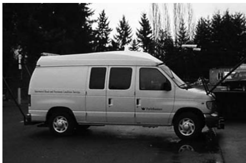
Washington State DOT uses automated data collection van (left) that travels at highway speeds collecting video images of the pavement surface (three samples below), as well as measurements of pavement rutting, wear, and smoothness.
