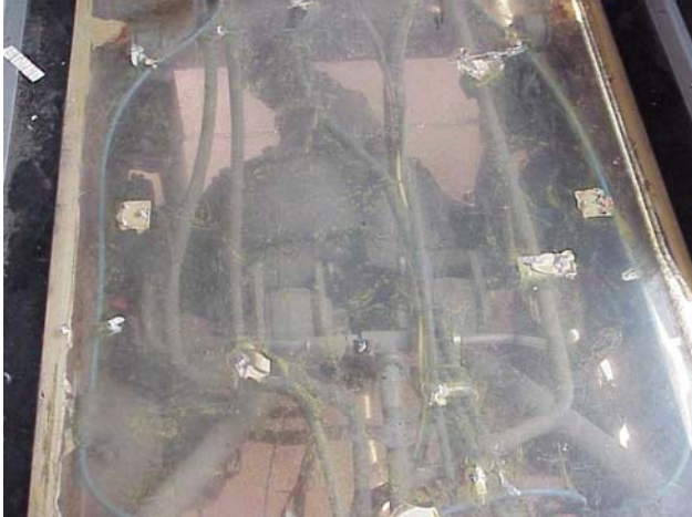
FIGURE 2 Plexiglas floor on training bus allows students to see components from inside the vehicle (source: DART).
