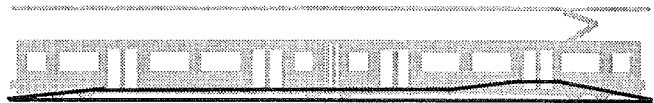
Figure 6.22 Profiled light rail platform Provides two steps into all doors, except the front door which is wheelchair accessible. All slopes are a maximum of 8.5° to meet ADA requirements. Most of the platform is only slightly higher than a sidewalk. Additional details on light rail wheelchair facilities with city specific information are contained in Chapter Eight, Light Rail Capacity Determination .
