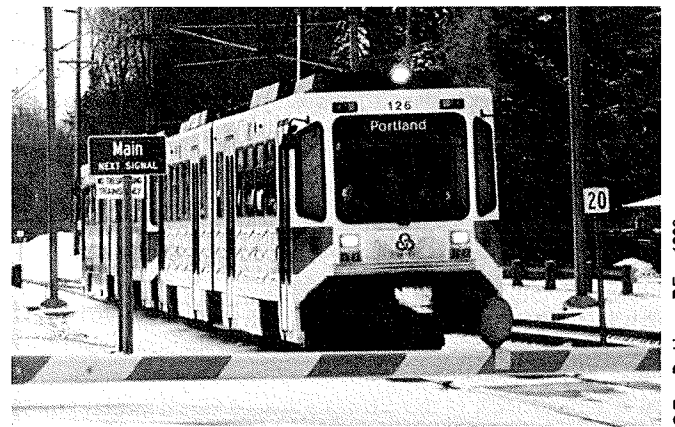
Figure 8.3 Tri-Met light rail train approaching an angled gated crossing (Note the gate is across the highway). The potential delay to cross traffic at these crossings is almost three times longer than with the 100% pre-empted signalized intersections closer to downtown. At higher train frequencies these occupancy times will become unacceptable and signalized intersections would be required—potentially reducing light rail speeds—but not the light rail capacity as the crossing occupancy time is well within a normal green phase.
