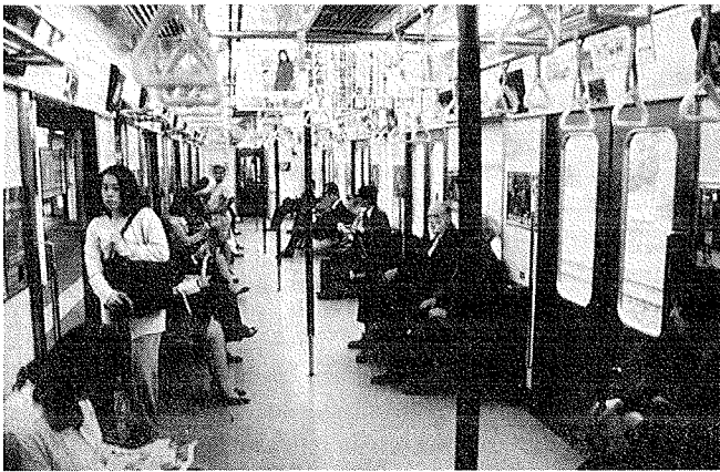
Figure 6.18 JR East high capacity car with six double doors and longitudinal seats that are locked up against the wall in the morning peak. The small number of seats are automatically unlocked at about 10.00h.
