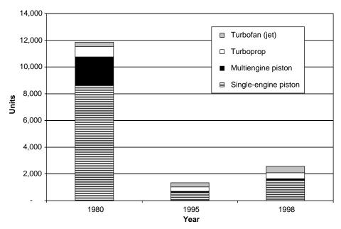
Figure 2-1 Shipments of new general aviation aircraft in the United States from domestic and foreign manufacturers, 1980, 1995, and 1998 (GAMA 1999b).
