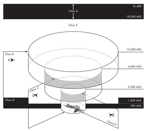
**Figure 2-2 Airspace structure in the United States** (see text for definitions of airspace Classes A through G) (FAA 2000a). Note: AGL = above ground level; FL = flight level; MSL = maximum sea level.
