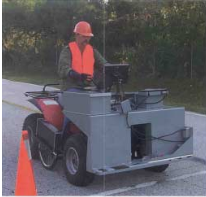
Figure 23. ATV configured single-track profiler – ICC.
