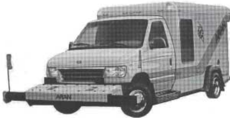
Figure 17. Roadware laser SDP profiler.
