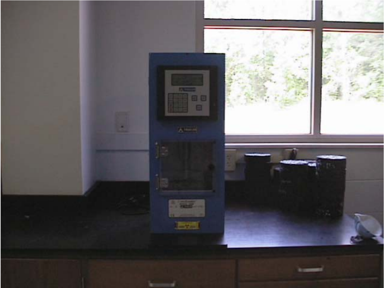
Figure 4: Gamma Ray Device (CoreReader)
