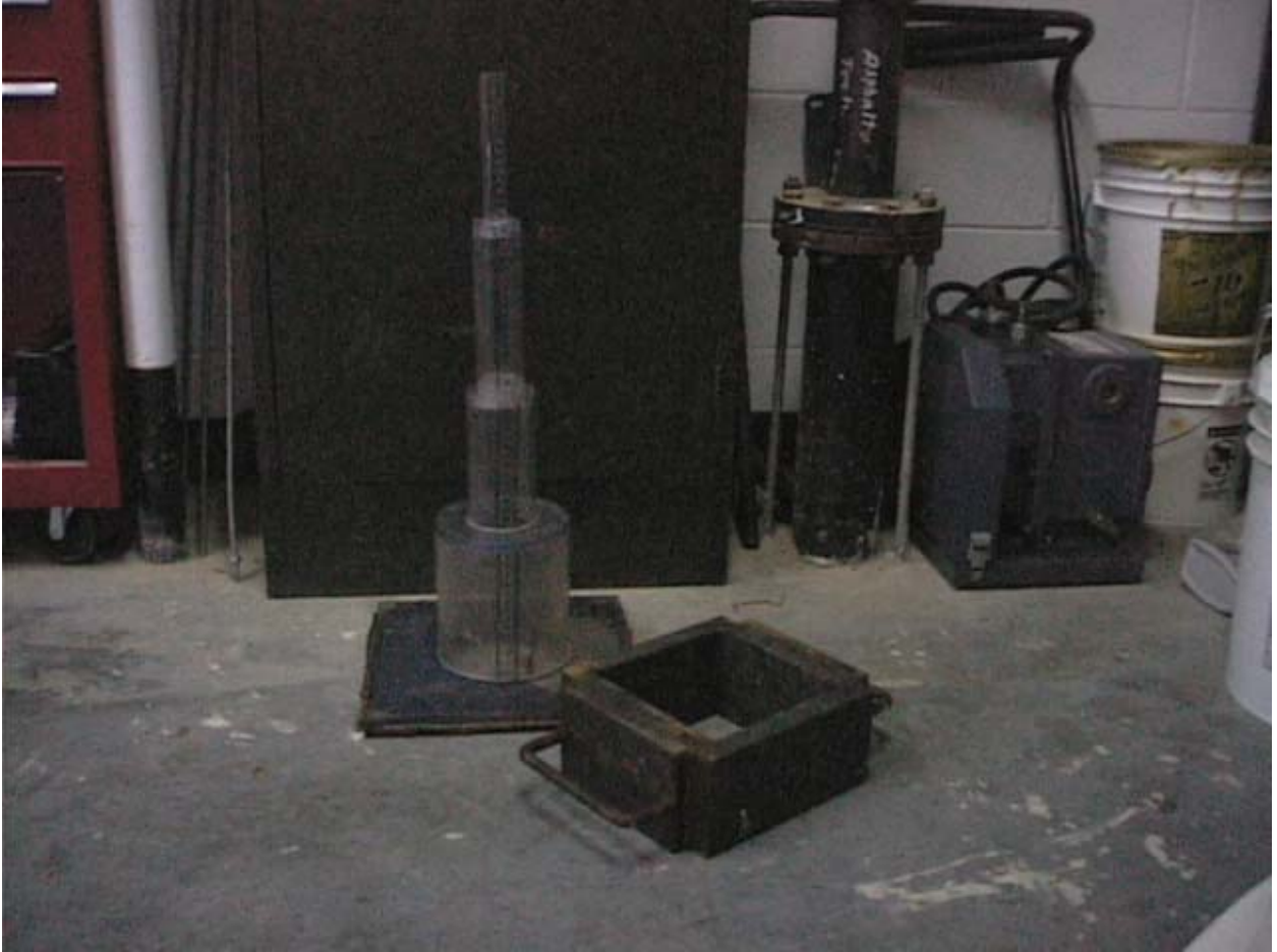
Figure 6: Field Permeability Device
