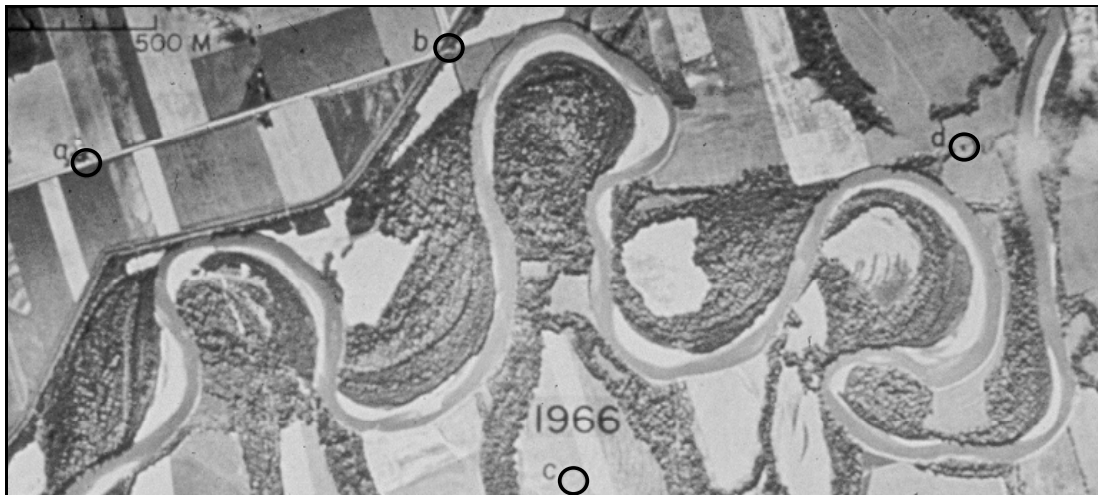
Figure 35. Aerial photo of a site on the White River in Indiana showing the four registration points common to the 1937 aerial photo in Figure 34.
