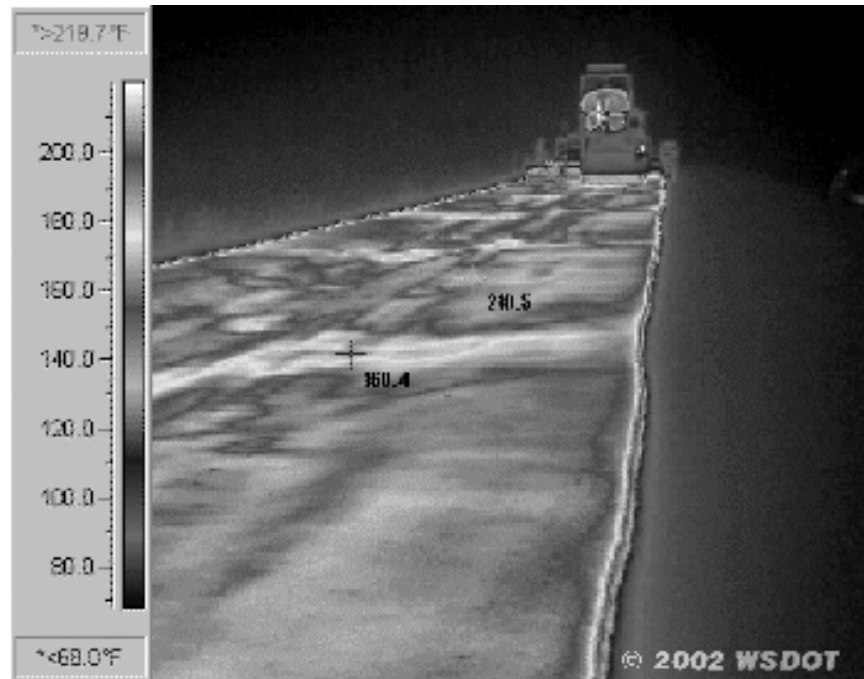
FIGURE 2 Thermal image of pavement with end-truck segregation.
