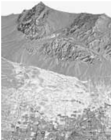
FIGURE 7 Fusion of ERS-2 satellite data (the background image) with ERS-1 data taken 3 years earlier (interferogram), both superimposed on TM 30-m data sharpened with SPOT 10-m panchromatic data. The interferogram shows an area of subsidence (at the millimeter level) near Las Vegas, Nevada, caused by groundwater withdrawal during the 3-year interval. (From Professional Surveyor , Oct. 1999.)
