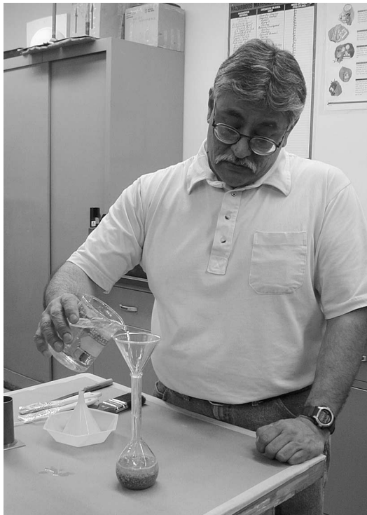
FIGURE 1 KT-50 is a simple method for determining the U-value or percentage of air voids in loosely compacted fine aggregates; the test can be performed in the field.
