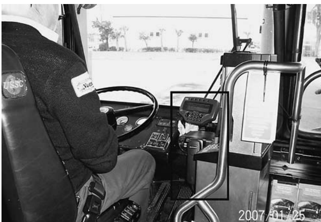
FIGURE 1 Typical fixed-route operator area with an AVL system (black box) (Courtesy: Doug Parker, TranSystems).
