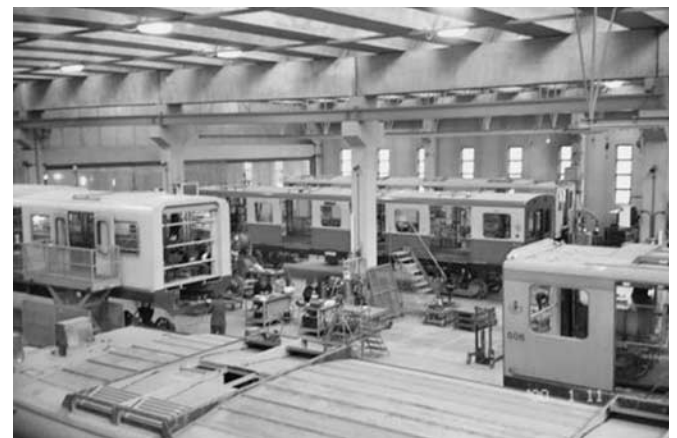
Figure 2 Car remanufacturing with new articulation in Milan.
