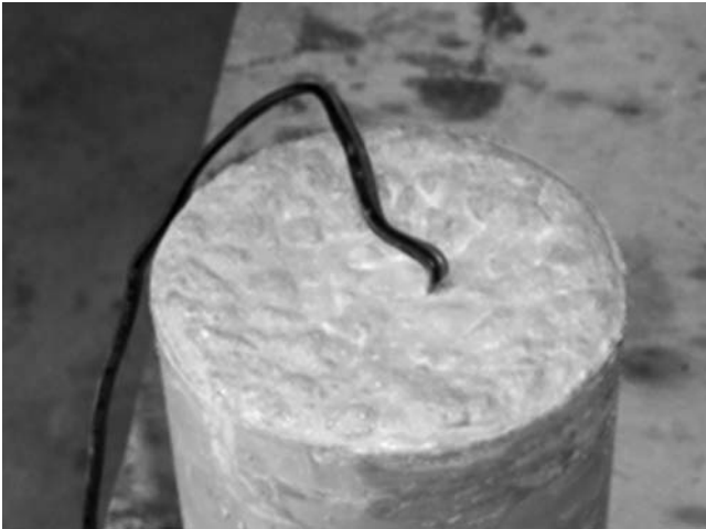
FIGURE 32 Sensor/logger encased in test cylinder.
