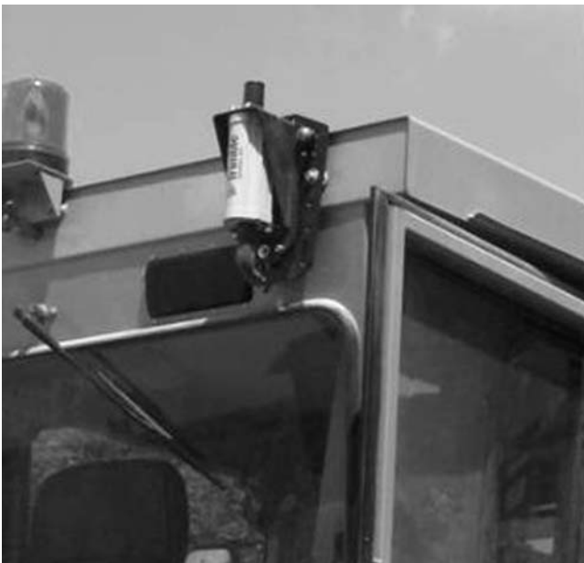
FIGURE 9 Cab-mounted GPS receiver (Courtesy: McAninch Corporation).
