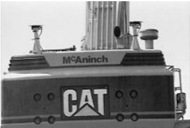
FIGURE 13 Dual GPS antennae on excavator counterweight (Courtesy: McAninch Corporation).
