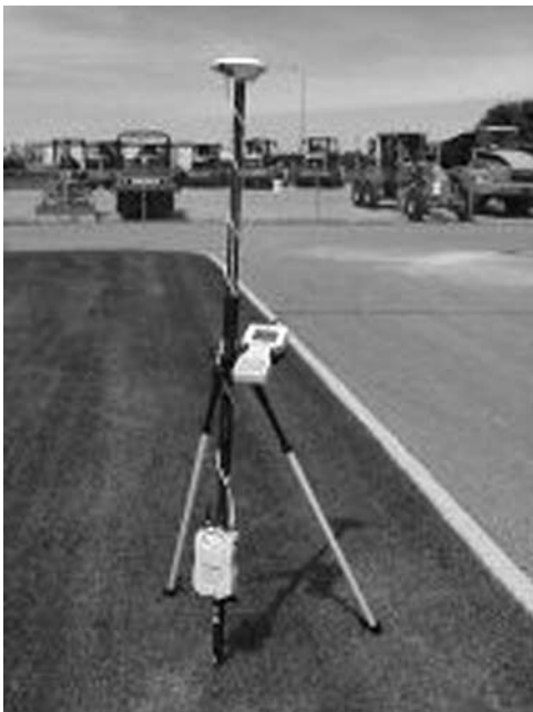
FIGURE 5 GPS antennae, receiver, and HHC tripod (Courtesy: McAninch Corporation).
