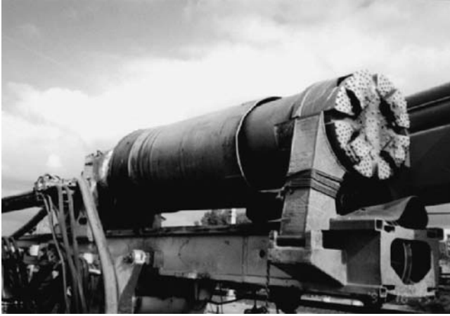
FIGURE 55 Downhole hammer tool for drilling in hard rock.
