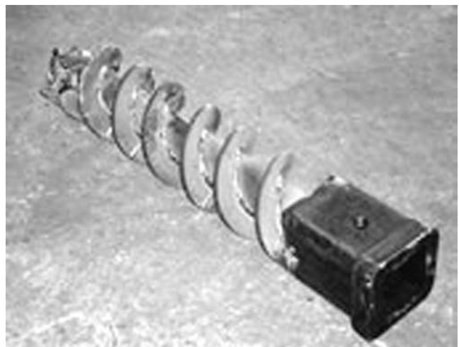
FIGURE 51 Small diameter rock auger for creating a pilot hole.
