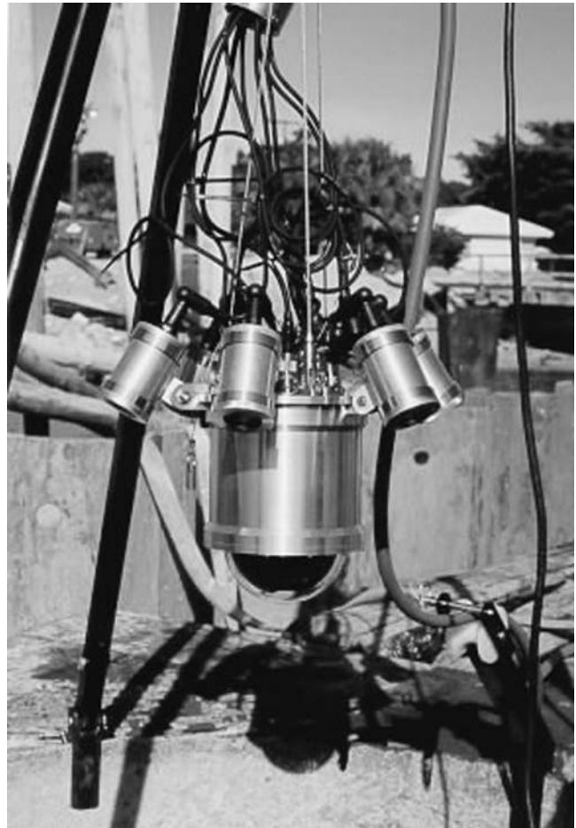
FIGURE 78 Shaft inspection device or SID.
