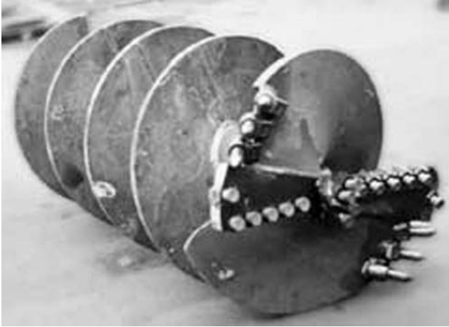
FIGURE 52 Rock auger with conical teeth and rotating cutters (Courtesy: V. Jue, Champion Equipment, Inc.).
