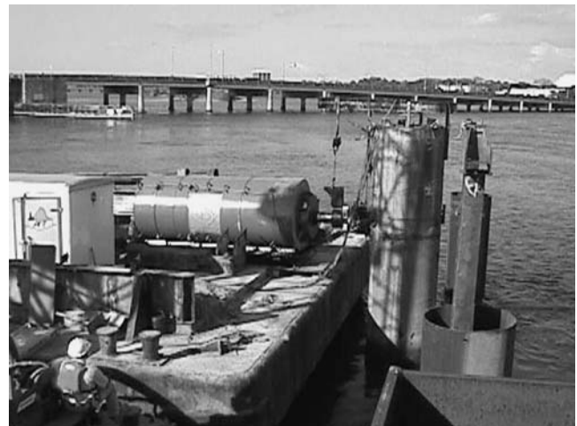
FIGURE 74 Lateral STN load test (Courtesy: L. Fontaine).
