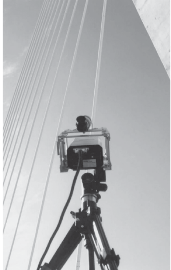
FIGURE 58 Use of laser doppler vibrometer for stay cable vibration and force measurements.
