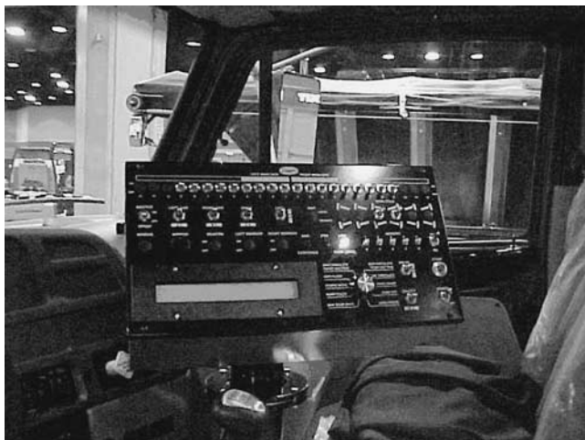
FIGURE 33 Computer rate control panel for binder distributor.
