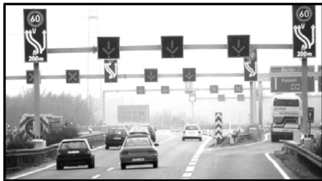
FIGURE 23 Tidal flow transition control devices, Hanover, Germany ( Source: Fellendorf et al. 2000).
