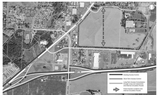
FIGURE 37 Highway 18/Highway 99W interchange access management plan.
