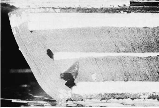
Figure 2.6. Damage due to cyclic shear displacements (from NCHRP Report No. 298).
