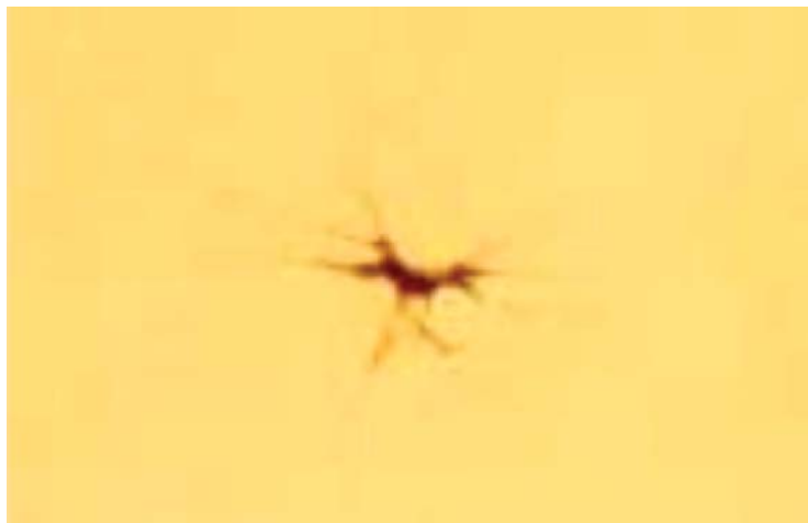
Figure 4.4.6-1 Example of impact-induced crack of facesheet.
