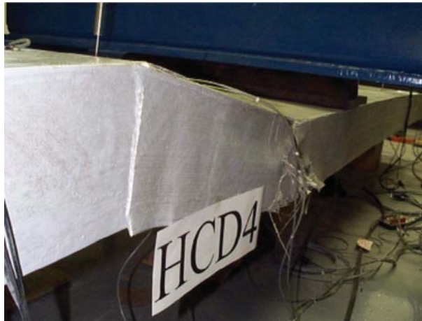
Figure 5.2.2.2-1 Foam sandwich deck failure under line load.
