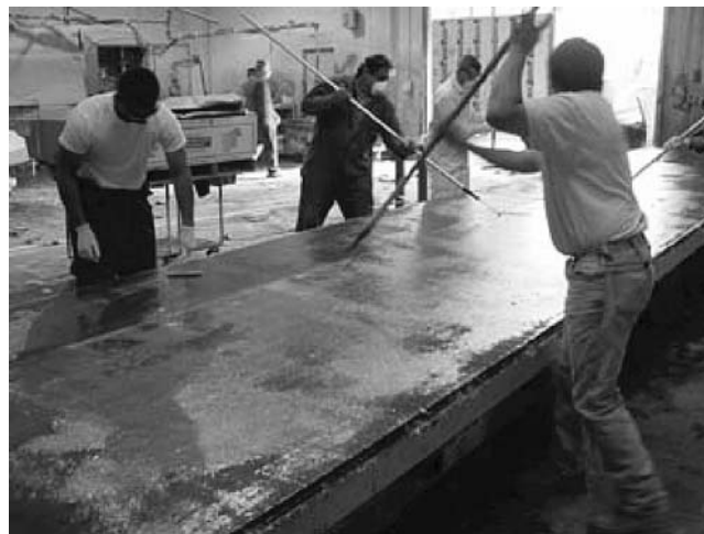
3.5.1-2 Hand lay-up operation: fabric saturation.
