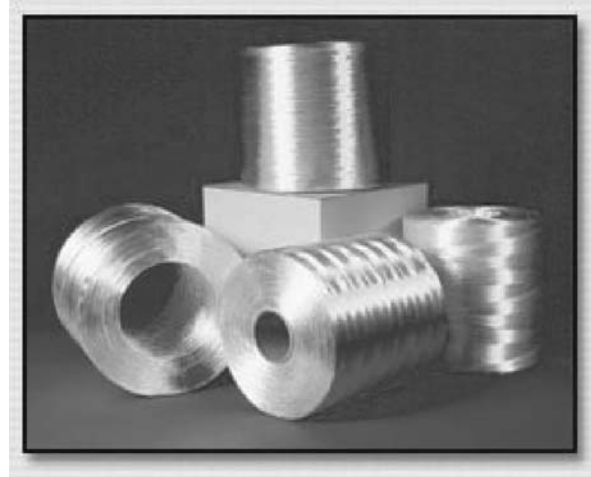
Figure 2.3.1.2-1 Spools of continuous fiberglass roving.
