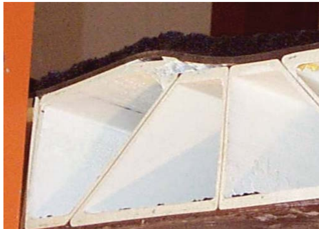
Figure 5.2.2.1-7 Tearing of core leading to facesheet buckling.
