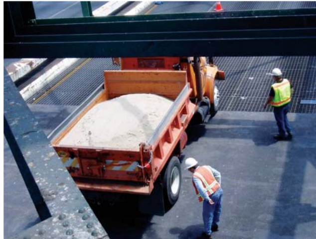
Figure 5.1.1-1 Dump truck placed on deck to reveal any cracks in FRP deck.
