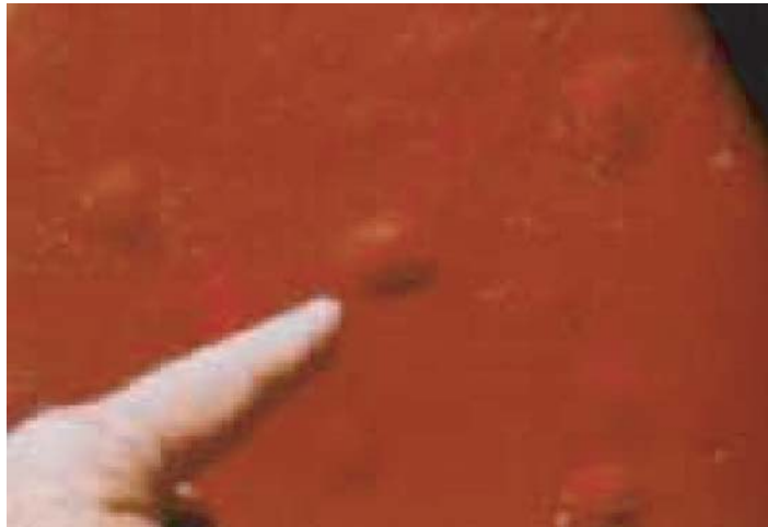
Figure 4.4.1-1 Blistering on a gelcoated or laminated surface.
