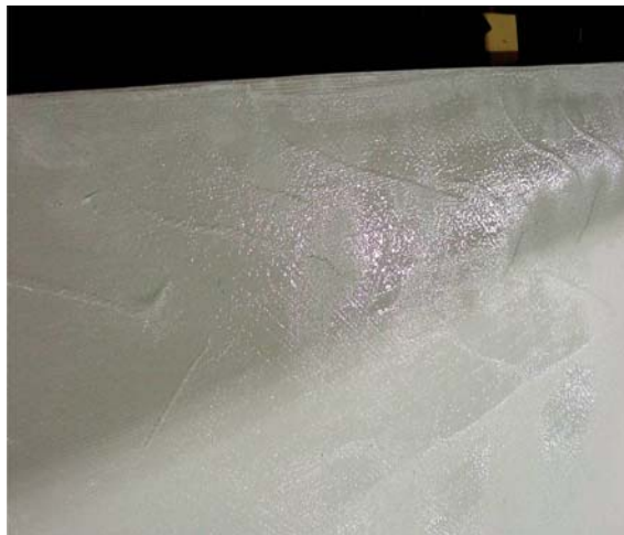
Figure 4.4.4-1 Fabric wrinkling in laminated facesheet.
