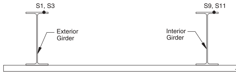
(b) Cross-sectional view showing the relative location for strain gages S1, S3, S9, and S11
